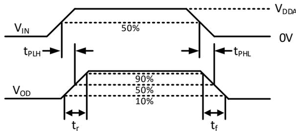
Figure 8-3 Driver propagation delays and rising/falling time
