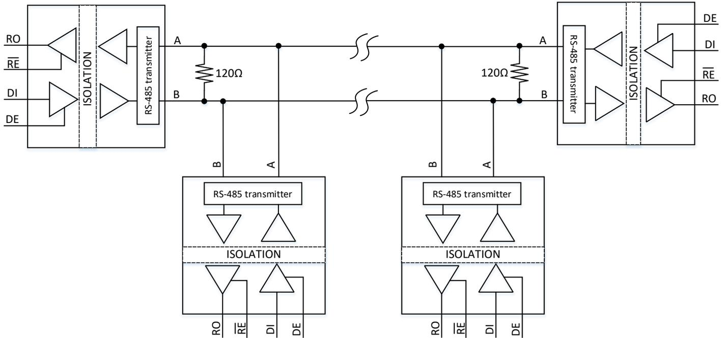
Figure 10-2 Typical isolated half-duplex RS485 application circuit
