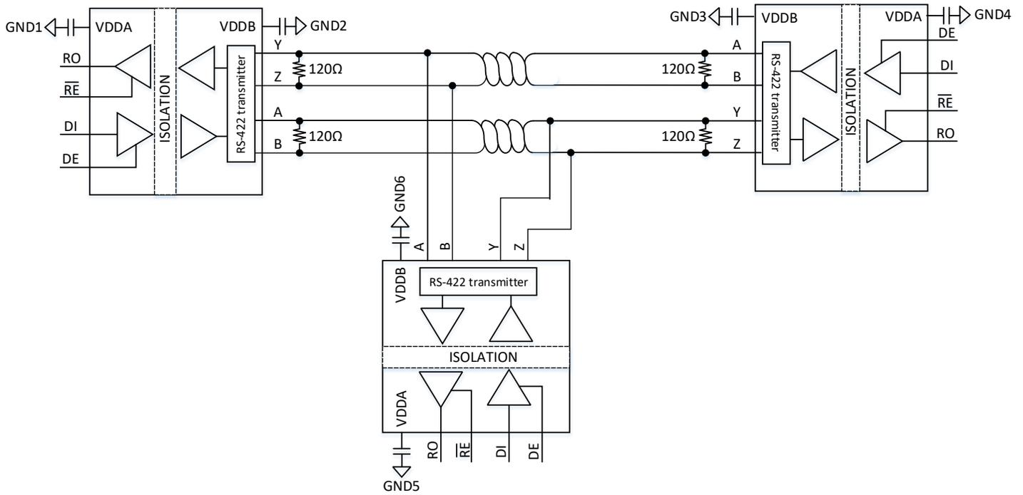
Figure 10-1 Typical isolated full-duplex RS422 application circuit
