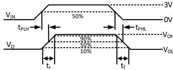
**Figure 8-5 Receiver propagation delays and rising/falling time**
